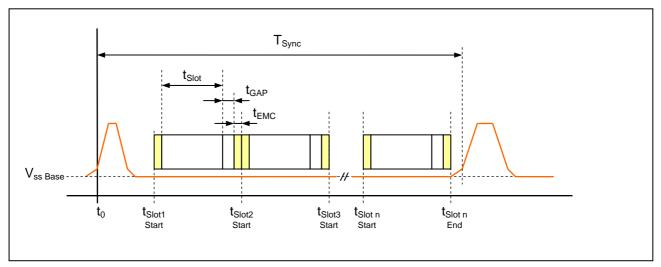
Figure 25 Timing of synchronous operation
