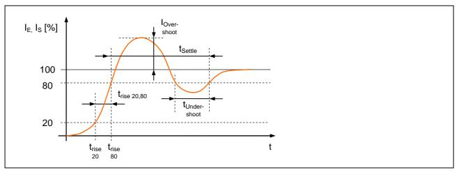
Figure 30 Test parameter sending current
