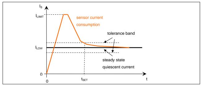
Figure 20 Current consumption during startup
