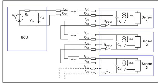
Figure 9 Synchronous Daisy Chain Bus (simplified schematic)
