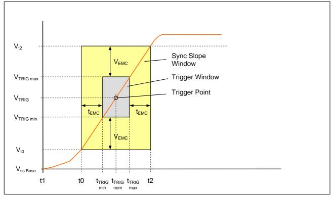
Figure 24 Trigger Point
