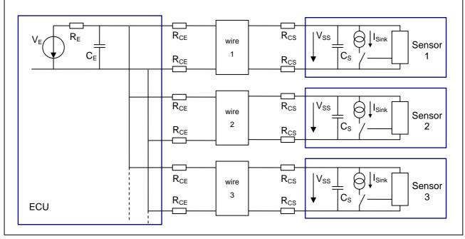
Figure 7 Synchronous Parallel Bus Mode (simplified schematic)
