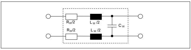
Figure 26 Supply line model for PSI5
