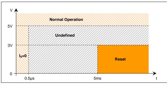
Figure 21 Undervoltage reset behaviour
