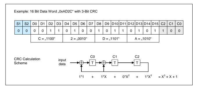
Figure 13 16 Bit Data word example with 3-Bit CRC
