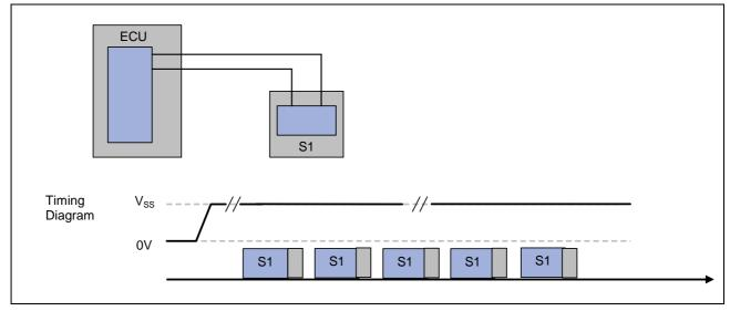
Figure 3 PSI5-A asynchronous point-to-point connection
