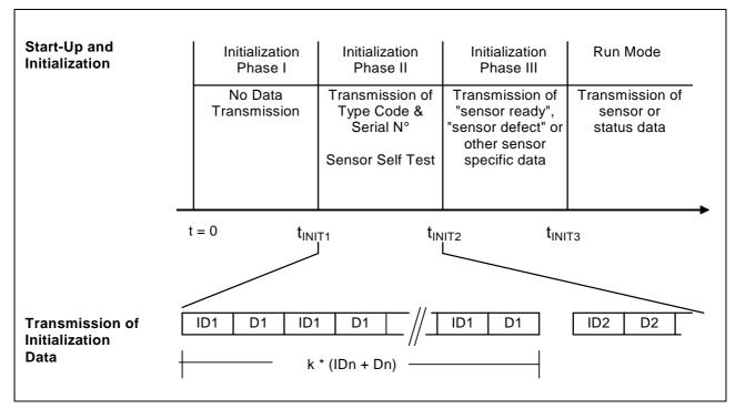
Figure 15 Initialization of the sensor
