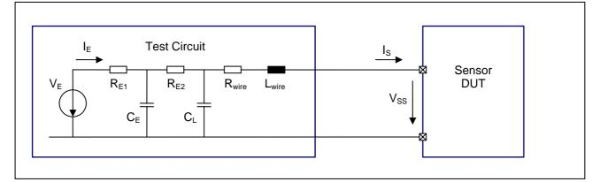
Figure 27 Reference test bench for sensor testing
