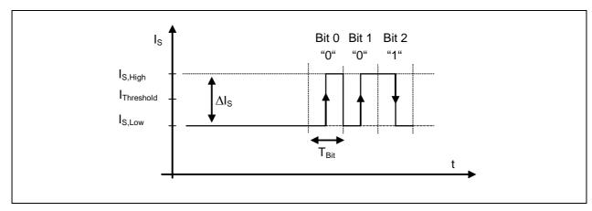
Figure 11 Bit encoding using supply current modulation
