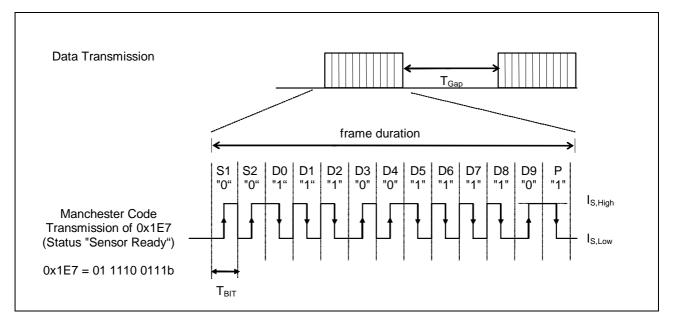
Figure 12 Example of a data frame with 10 data bits (D0-D9), 2 start bits (S1,S2) and one parity bit (P).
