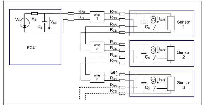
Figure 8 Example for a pass-through configuration (simplified schematic)
