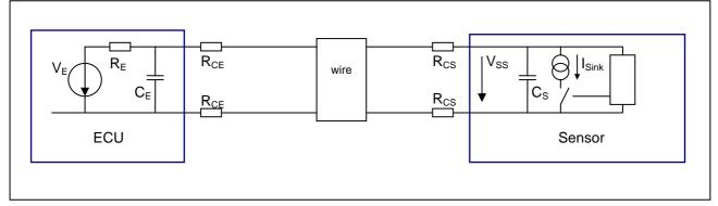
Figure 4 Single sensor configuration (simplified diagram)
