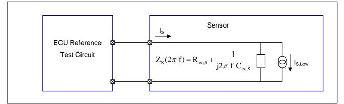
Figure 28 Reference circuit for sensor damping behaviour
