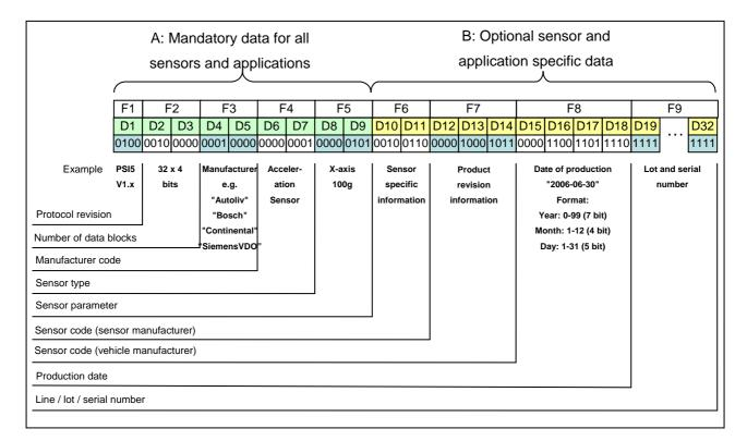
Figure 18 Initialization phase 2: Recommended Data Content
