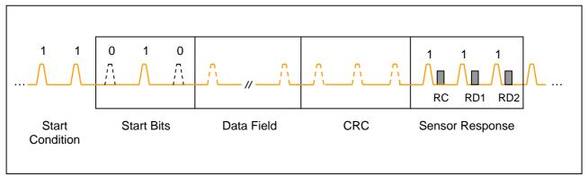
Figure 19 Data frame ECU to sensor communication
