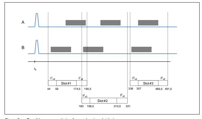
Possible message timing for overlapping slot timings Figure 3
