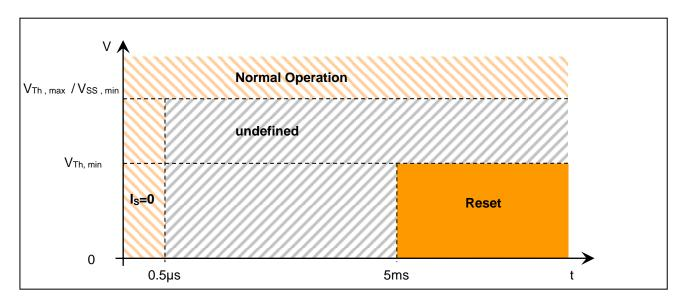
Figure 2 Undervoltage reset behaviour
