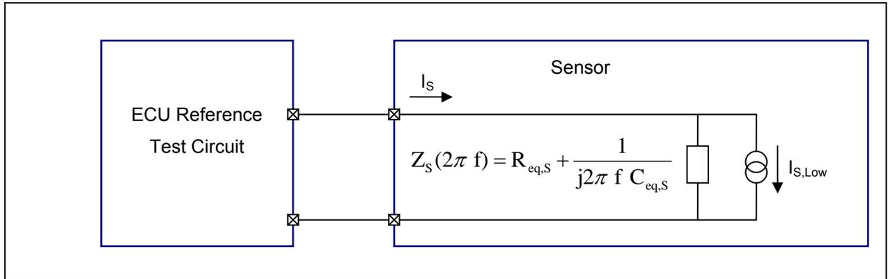
622 *Figure 38 Reference circuit for sensor damping behaviour*
