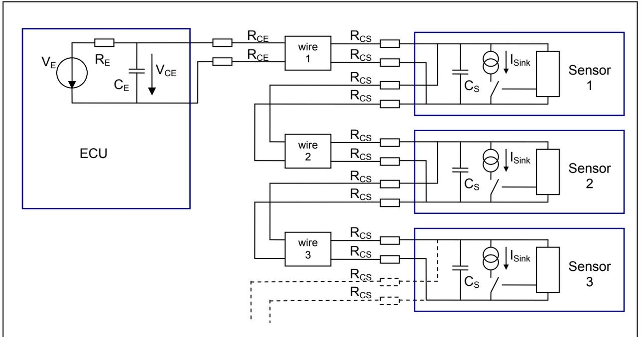
150            *Figure 11 Example for a pass-through configuration (simplified schematic)*
