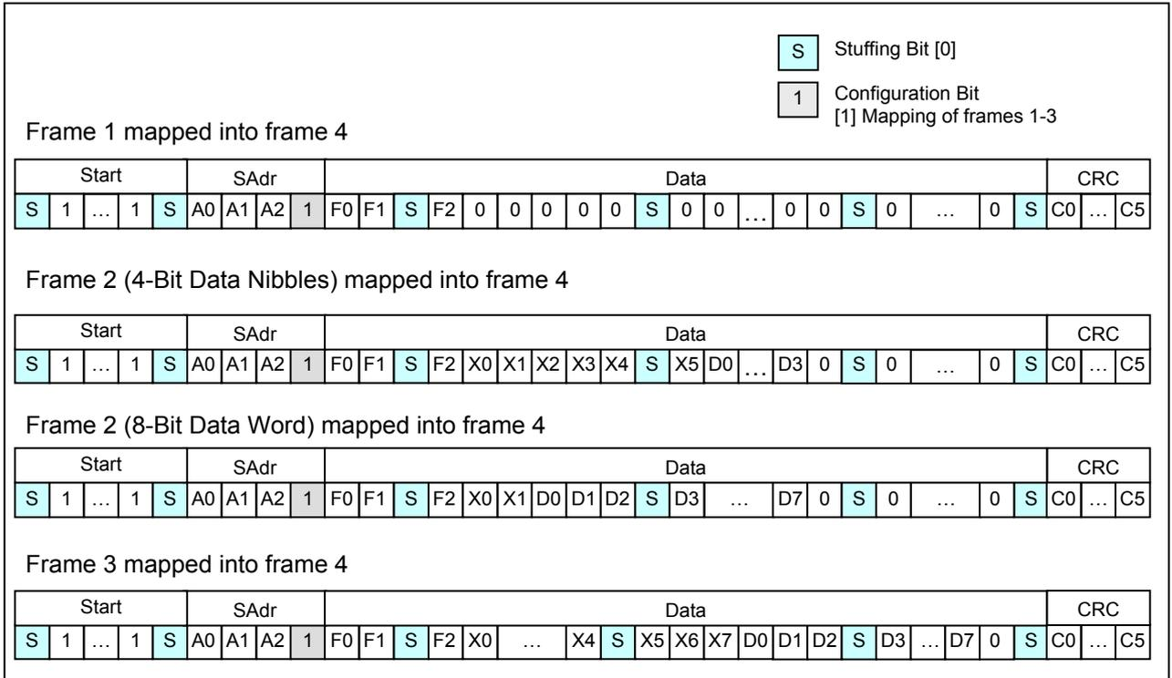
325 *Figure 27 Mapping of frames 1-3 into frame 4*
