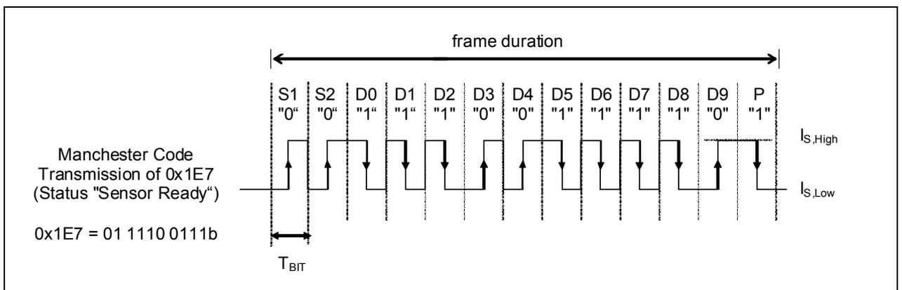
191 *Figure 15 Example of a data frame with 10 data bits (D0-D9), 2 start bits (S1,S2) and one parity bit (P).*
