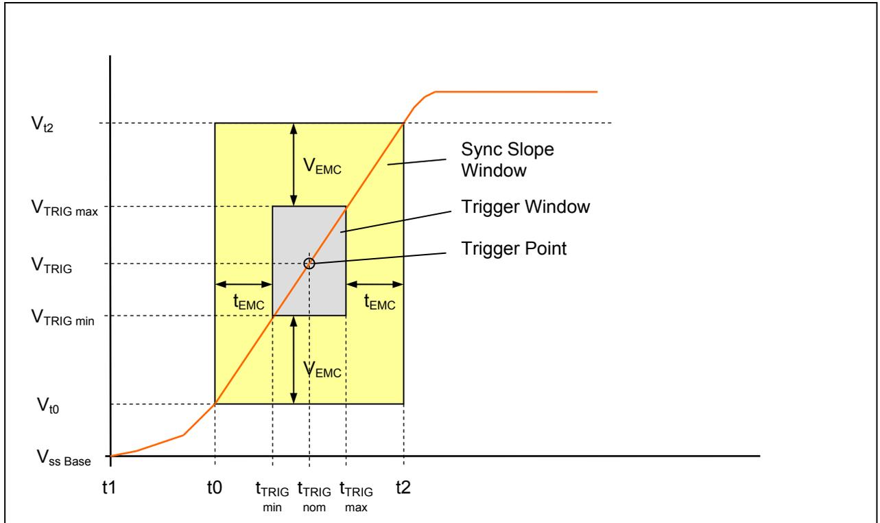
504 *Figure 34 Synchronization signal detection in the sensor*
