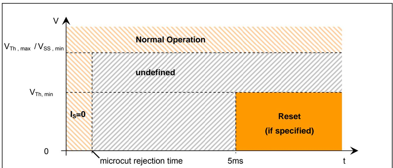
453 *Figure 31 Undervoltage reset behaviour*
