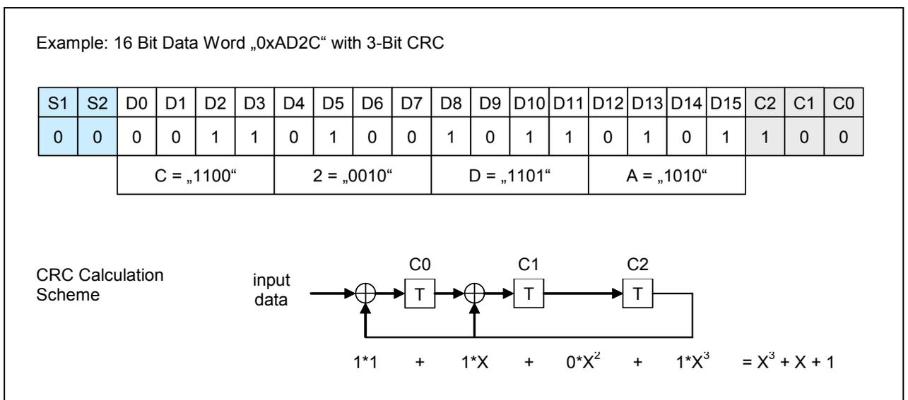
204 *Figure 16 16 Bit Data word example with 3-Bit CRC*
