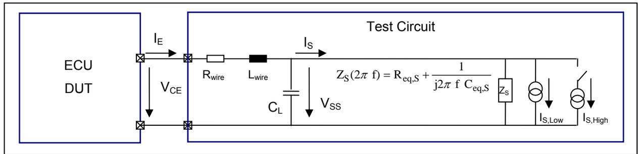
657 Figure 41 Reference test bench for ECU testing
