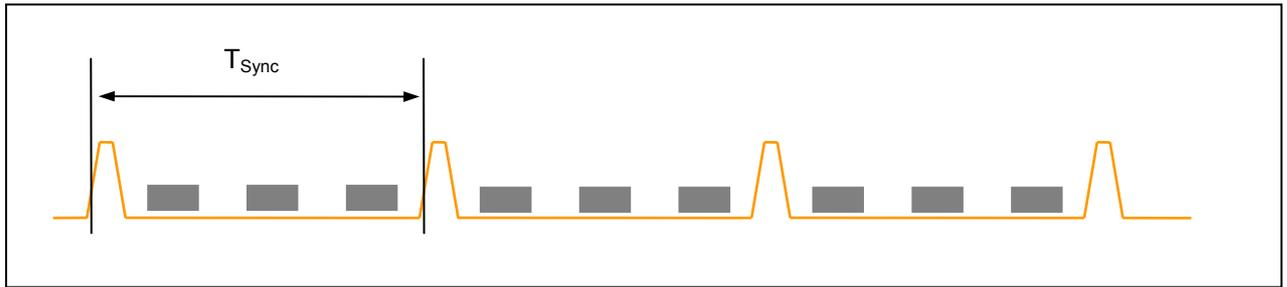
98 *Figure 5 Fixed time triggered synchronous operation*
