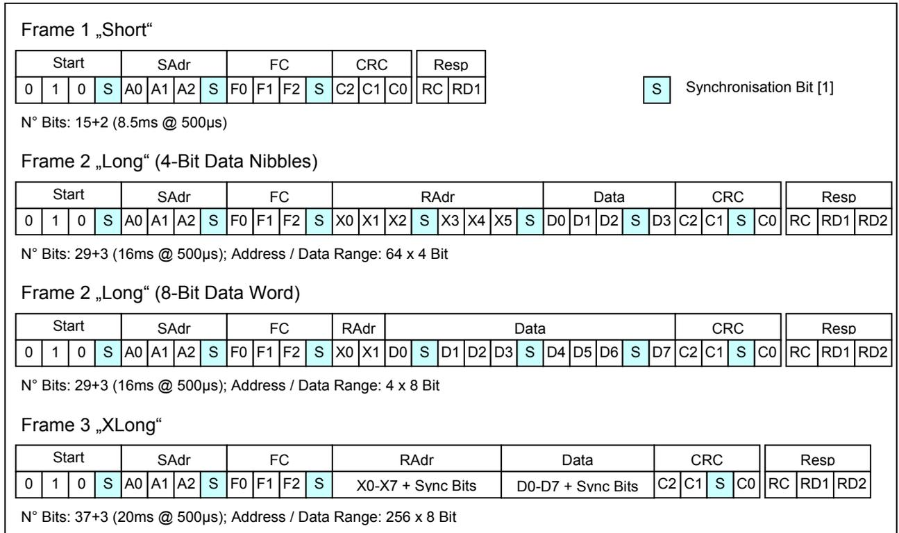
304 *Figure 24 Data frames 1-3 ECU to Sensor Communication*
