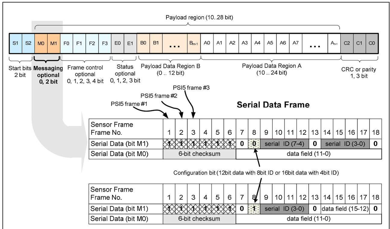
248 *Figure 19 Serial Data Frame generated by the two messaging bits of the sensor data frame (messaging*
