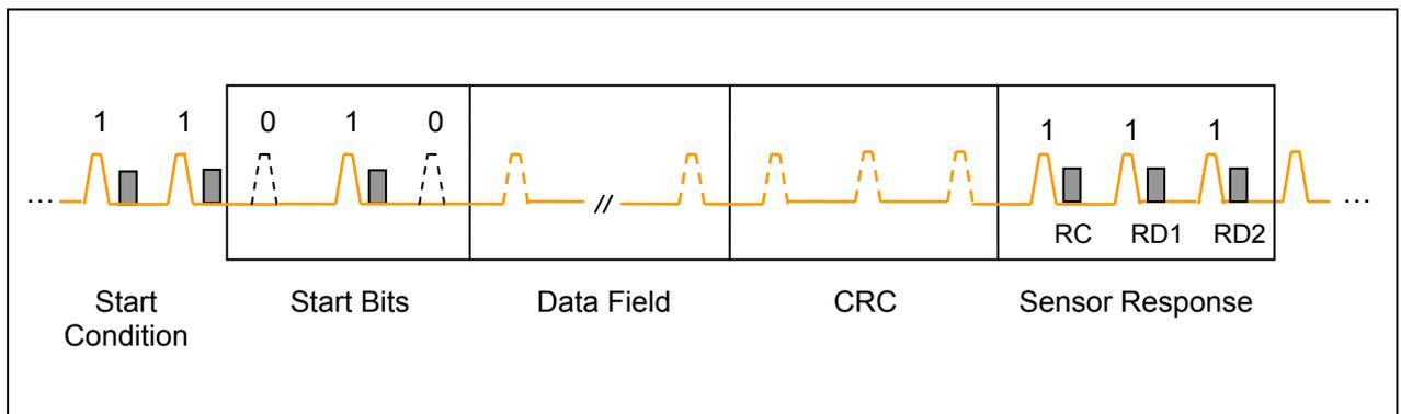
295 *Figure 23 Data frame ECU to sensor communication – e.g. Tooth Gap method applicable to frame*
