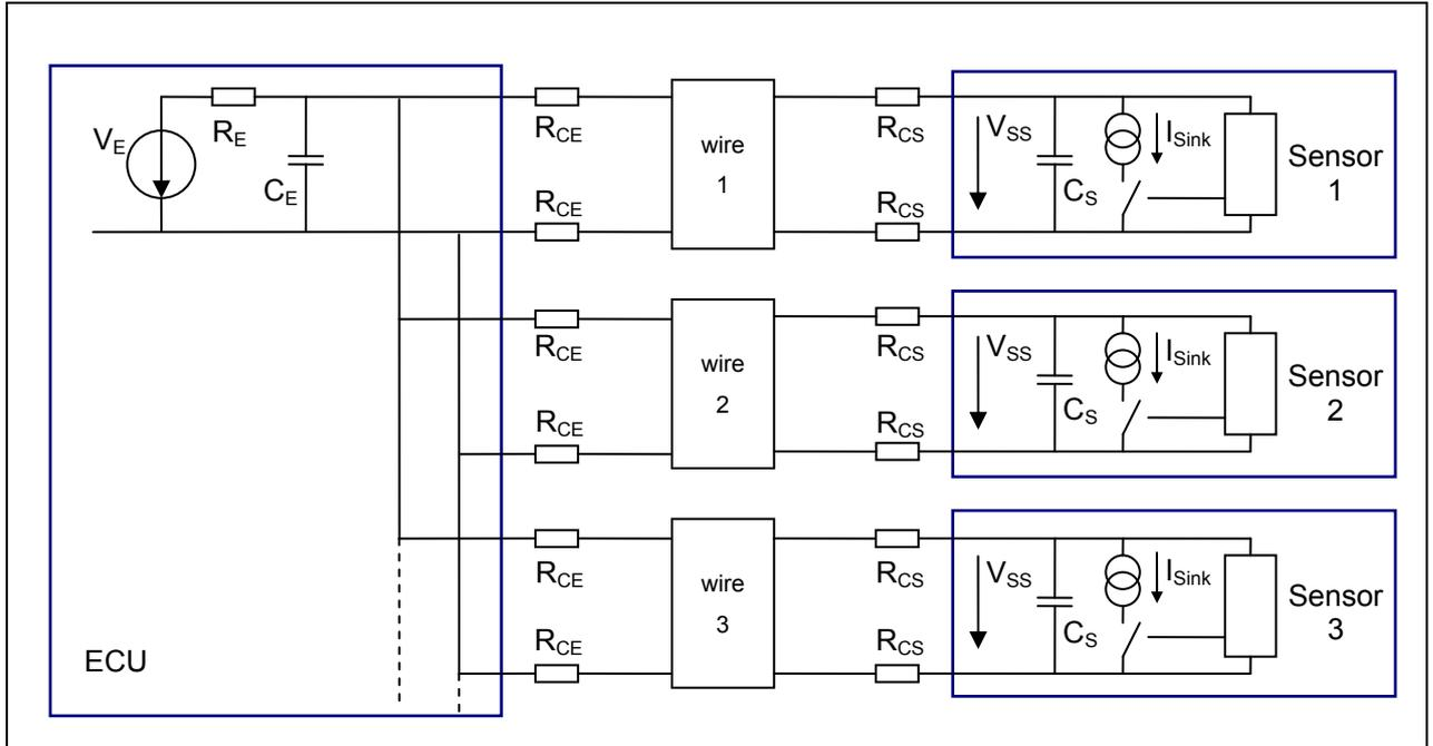
142            *Figure 10 Synchronous Parallel Bus Mode (simplified schematic)*
