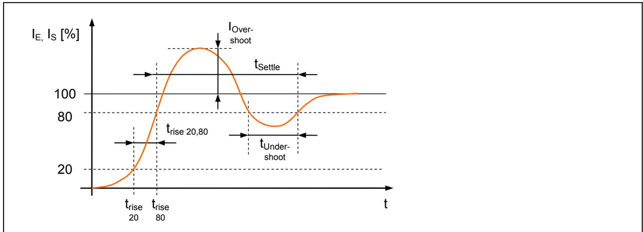
638 Figure 40 Test parameter sending current
