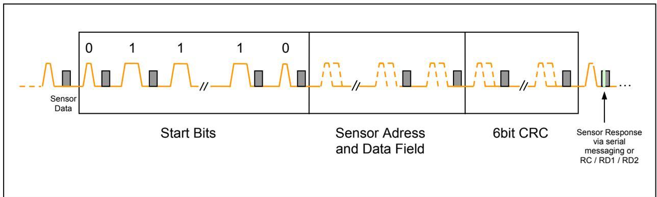
313 *Figure 25 Data frame ECU to Sensor Communication –e.g. Pulse width method with frame format 4*
