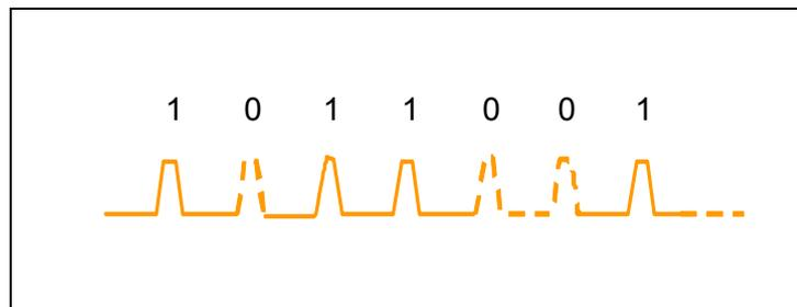
267 *Figure 21 Bit Encoding according to the Tooth Gap Method*
