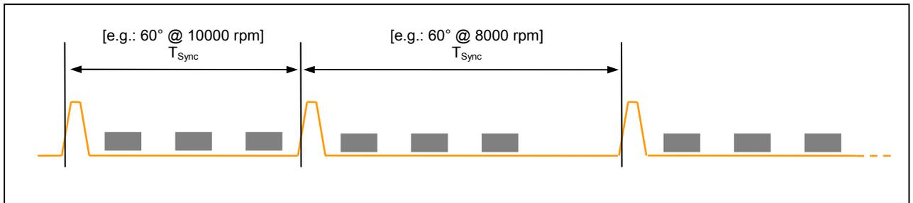
99 *Figure 6 Variable time triggered synchronous operation*
