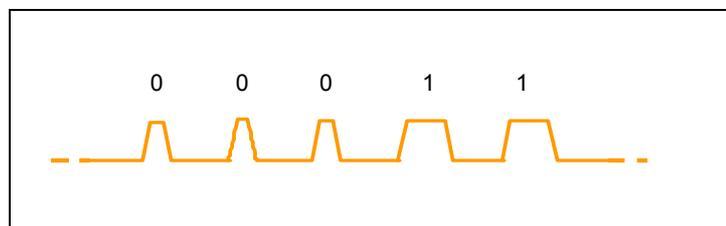
273 *Figure 22 Bit Encoding via Pulse width*
