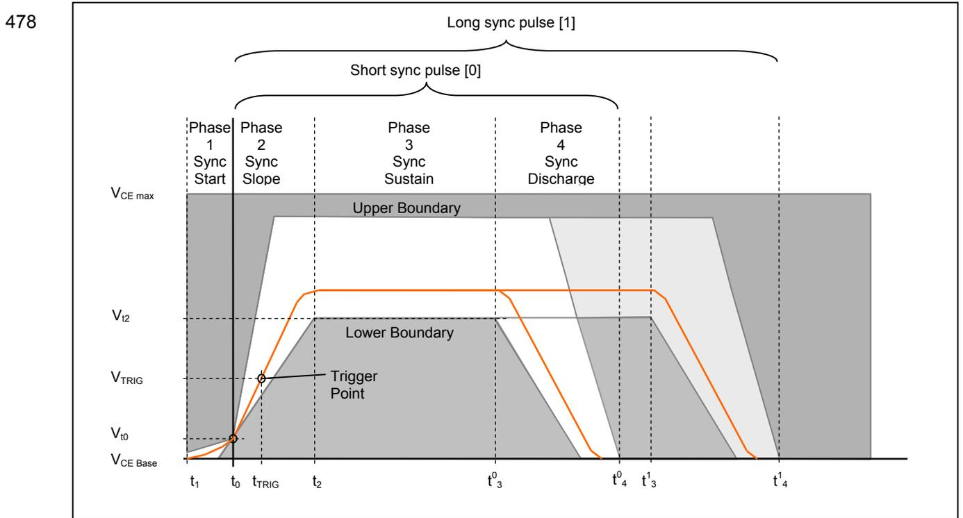
479 *Figure 33 Shape and timing of Synchronization Signal at Receiver*
