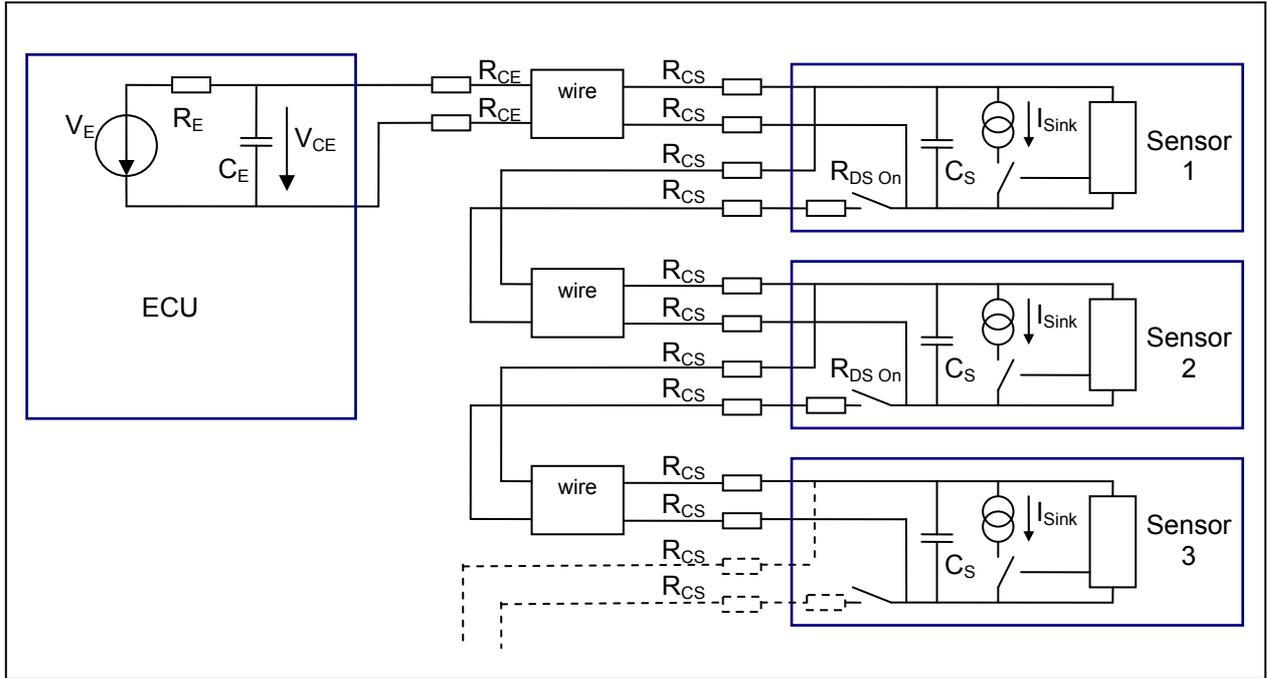
160 *Figure 12 Synchronous Daisy Chain Bus (simplified schematic)*
