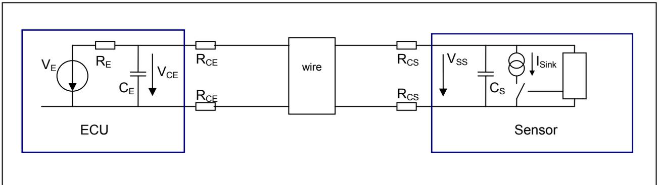
93 *Figure 4 Single sensor configuration (simplified diagram)*
