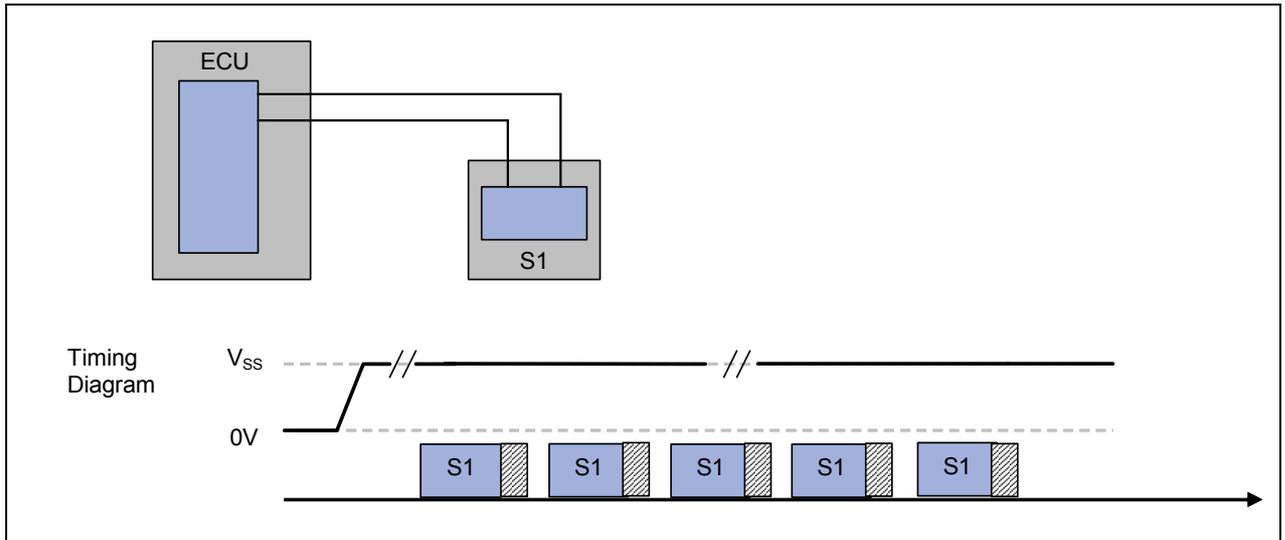
91 *Figure 3 PSI5-A asynchronous point-to-point connection*
