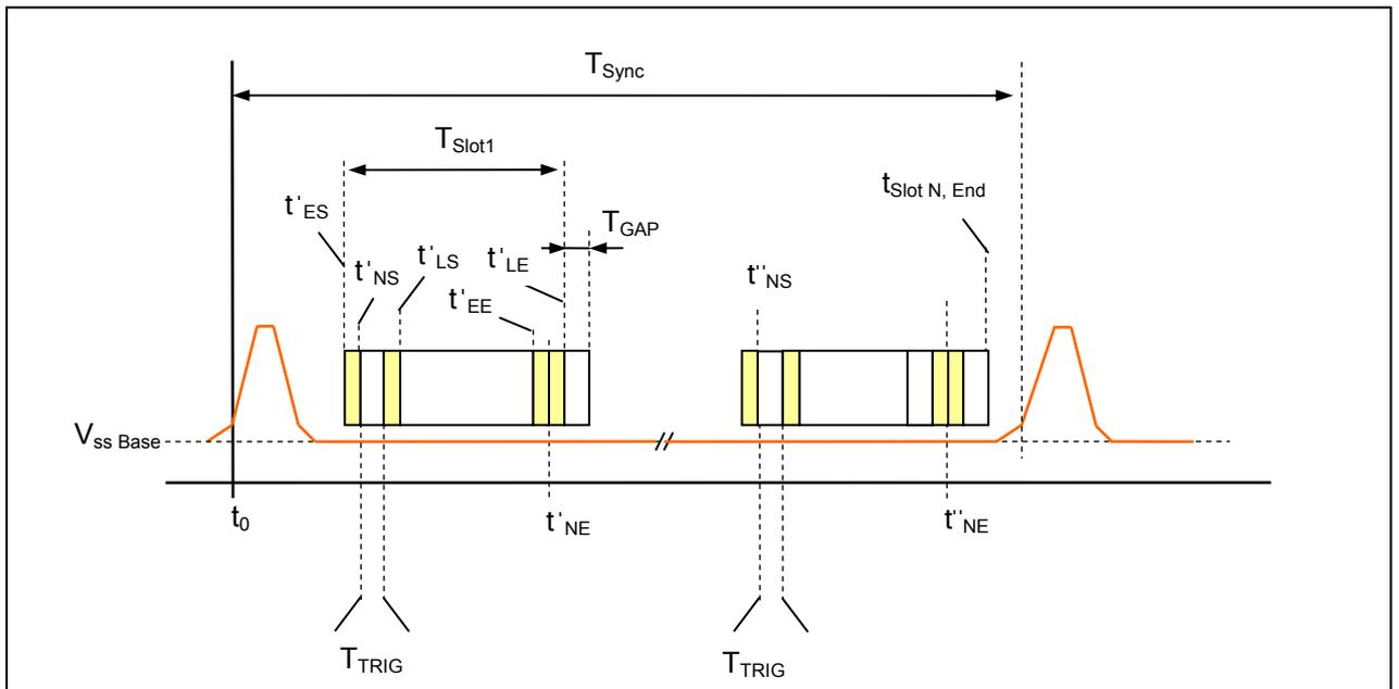
522 Figure 35 Timing of synchronous operation
