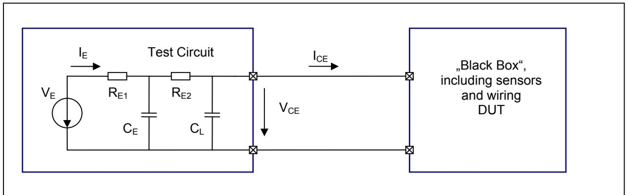
632    *Figure 39    Reference test bench for bus testing*
