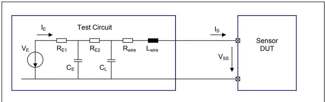
615 *Figure 37 Reference test bench for sensor testing*
