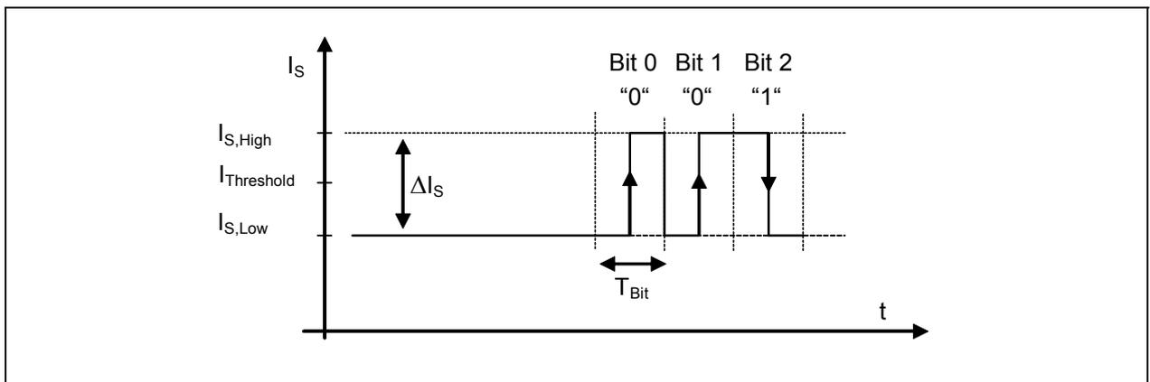
181 *Figure 14 Bit encoding using supply current modulation*
