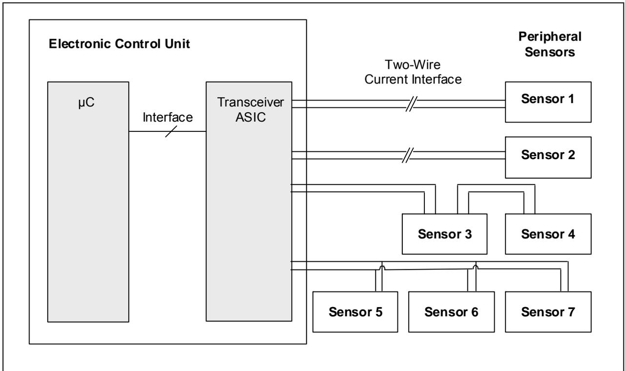
75 *Figure 1 Connection of peripheral sensors to an ECU (Example)*
