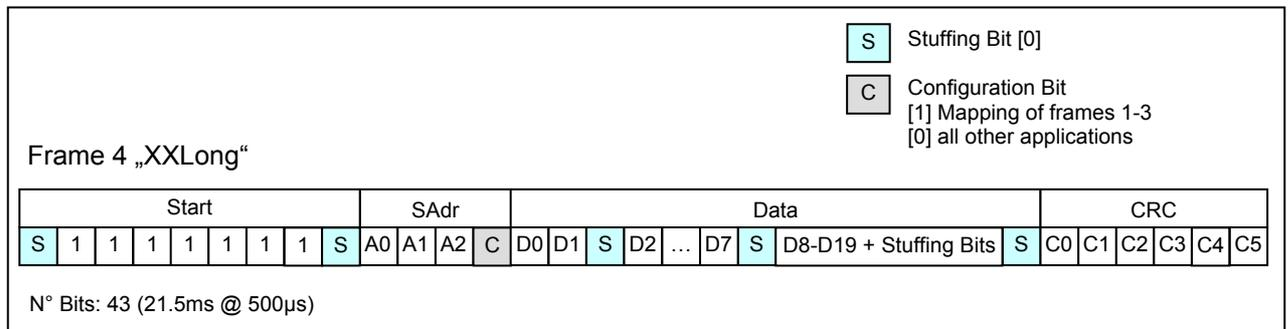
315 *Figure 26 Data frame4 ECU to Sensor Communication*
