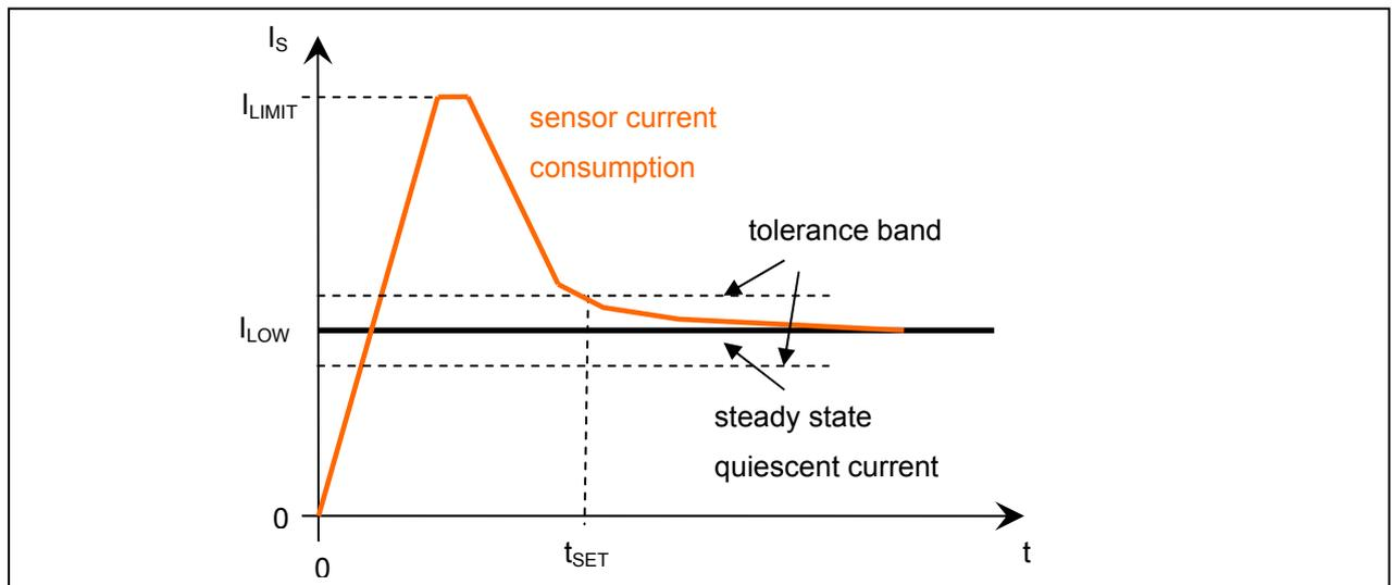
441 *Figure 30 Current consumption during startup*
